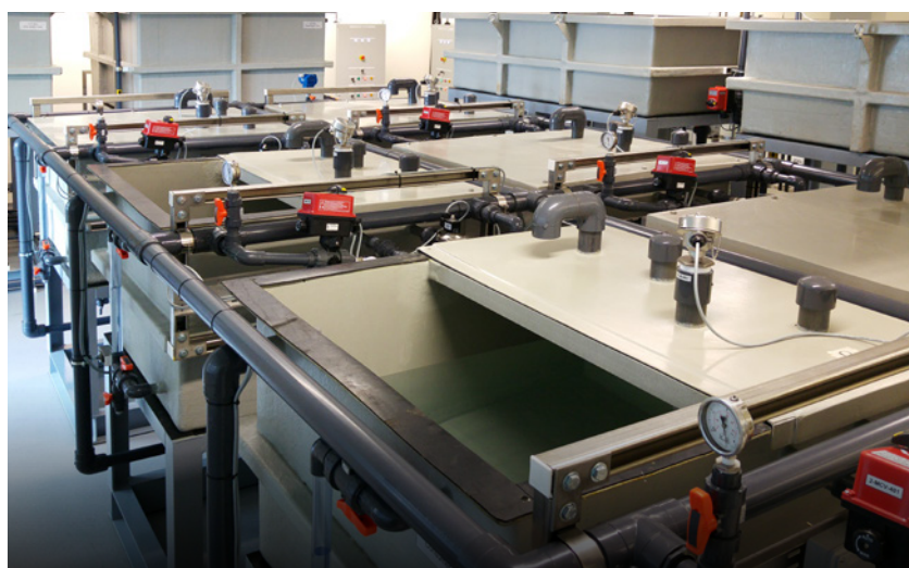
Bottom: Elevated reservoir tanks from the Water Distribution (WADI) test bed, extended from SWaT. Source: SUTD.
